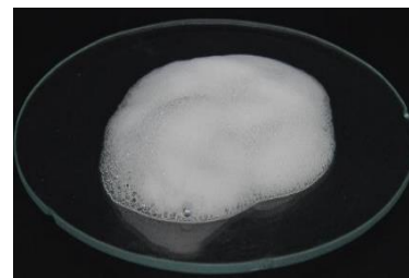
Water soluble silicone less foam with low density big and open bubbles
